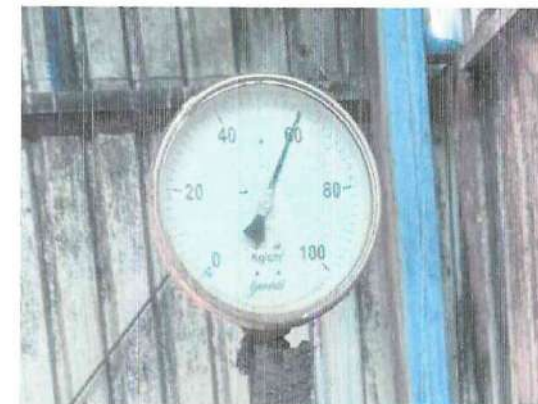
Hydrostatic test pressure 60 Barg. Holding 30 min.
